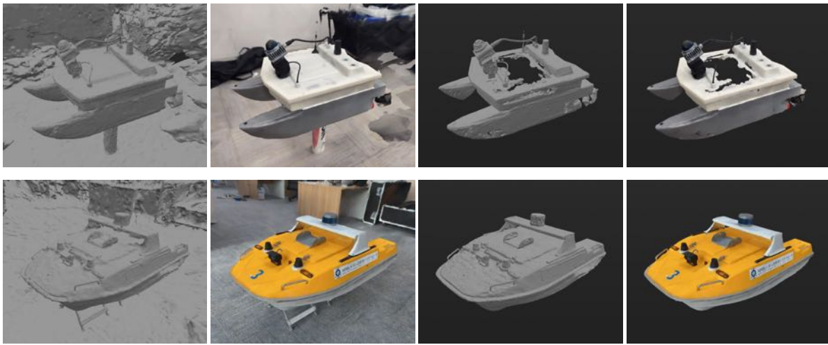
Figure 4.2: 3D USV Model (Upper row) and Target Model (Bottom row)
